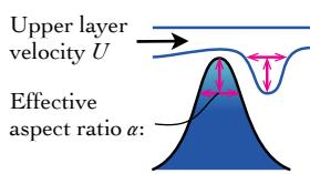
Fig. 5. Wave generation on the lee side of a tall sill
